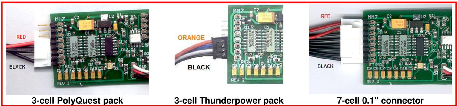
When plugged in, **MM7** will first "boot up" (**RED**-pause-**GREEN**-pause). The LED then will blink the cell count in **RED**. Finally, A crude indication of capacity is shown. Steady **GREEN** means full or almost full. Blinking **GREEN** indicates partially full, and **RED** means nearly empty. The LED shuts off after a few seconds.
