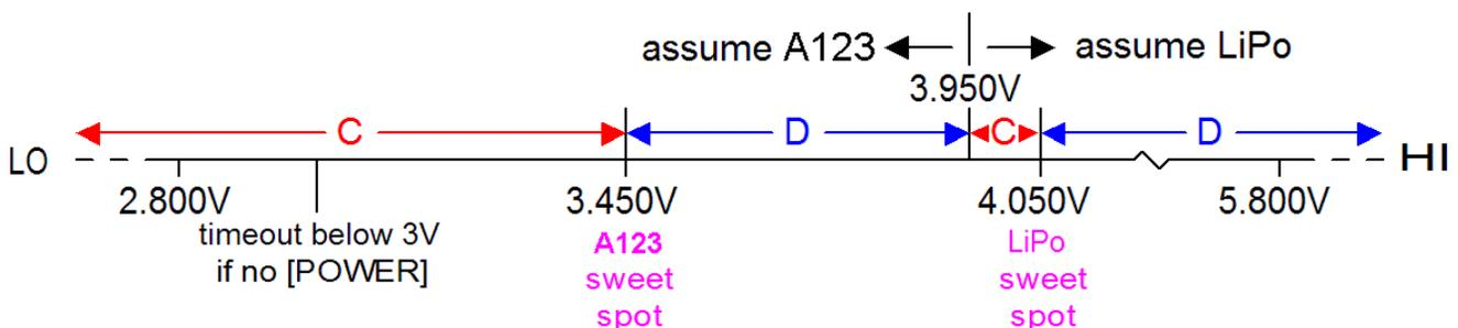
As the "sweet spot" (3.45V for A123, 4.05V for LiPo) is approached from either direction, the following displays are used:
